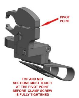
STEP 1 - Loosen the clamp screw so the top section seperates from the mid section. This will provide the necessary clearance to slide the mount over the mirror stem as shown above. Adjust the mirror paralell to the windshield and slightly upward for ease of installation.
