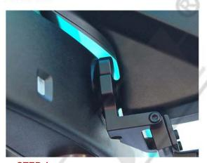
**STEP 4 -** Rotate the mount so it is parallel with the bottom of the mirror. Tighten the clamp screw untill the mount is securely attached to the mirror stem. Do not over tighten the clamp screw.
