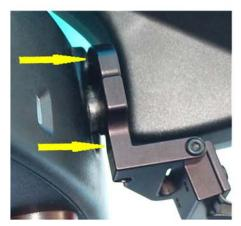
STEP 3 - Position the mount as far forward as you can. Tighten the clamp screw untill the Top and Mid Sections are slightly snug around the mirror stem. You should still be able to rotate the mount.
